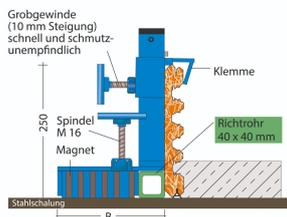
The MK 3 magnetic clamp is used to attach formwork profiles to steel formwork. They are used for shuttering balcony upstands, wall and ceiling end formwork as well as door and window recesses. The standpipe is firmly welded. Profiles up to a width of 250 mm can be clamped in the magnetic clamp. The uprights can also be supplied in a higher version on request.
