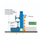
The MK 3 magnetic clamp is used to attach formwork profiles to steel formwork. They are used for shuttering balcony upstands, wall and ceiling end formwork as well as door and window recesses. The standpipe is firmly welded. Profiles up to a width of 250 mm can be clamped in the magnetic clamp. The uprights can also be supplied in a higher version on request.
