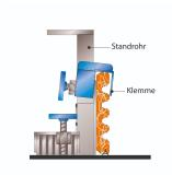
The MK 4 magnetic clamp is used to attach shuttering profiles to steel formwork. They are used for shuttering balcony upstands, wall and ceiling end formwork as well as door and window recesses. The standpipe is inserted into the magnetic element and can be pulled out. This makes it possible to remove the surface of the concrete component without hindrance. Profiles up to a width of 250 mm can be clamped in the magnetic clamp. The standpipes can also be supplied in a higher version on request.
