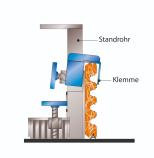
The MK 4 magnetic clamp is used to attach shuttering profiles to steel formwork. They are used for shuttering balcony upstands, wall and ceiling end formwork as well as door and window recesses. The standpipe is inserted into the magnetic element and can be pulled out. This makes it possible to remove the surface of the concrete component without hindrance. Profiles up to a width of 250 mm can be clamped in the magnetic clamp. The standpipes can also be supplied in a higher version on request.
