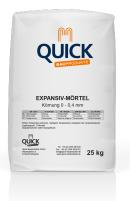
The EM 0-0.4 E1 expansive mortar is used to seal clamping points and for mortaring cavity wall joints. It has a very high adhesive strength. The mortar does not shrink but retains its volume and does not break away during hardening. It is pressed into the holes or joints using mortar presses. The fine grain size ensures that the surface can be removed smoothly. The mortar can also be pumped and installed using a suitable pump.
