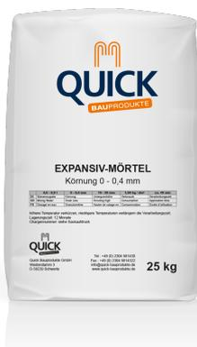
The EM 0-0.4 E1 expansive mortar is used to seal clamping points and for mortaring cavity wall joints. It has a very high adhesive strength. The mortar does not shrink but retains its volume and does not break away during hardening. It is pressed into the holes or joints using mortar presses. The fine grain size ensures that the surface can be removed smoothly. The mortar can also be pumped and installed using a suitable pump.
