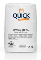
The EM 0-0.4 E1 expansive mortar is used to seal clamping points and for mortaring cavity wall joints. It has a very high adhesive strength. The mortar does not shrink but retains its volume and does not break away during hardening. It is pressed into the holes or joints using mortar presses. The fine grain size ensures that the surface can be removed smoothly. The mortar can also be pumped and installed using a suitable pump.
