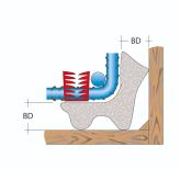
The Supo Duo is mounted on reinforcement cages in the stirrup corner area. It holds the concrete cover in two directions. Installation is possible on reinforcement  $\emptyset$  3-18 mm. The Supo Duo can also be supplied with 2 clamps as an option. Thanks to the specially designed clamp shape, the Supo clamps optimally to the reinforcing steel. Fast installation is guaranteed.
