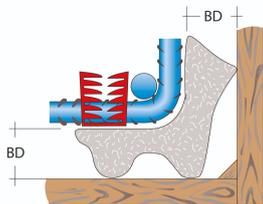
The Supo Duo is mounted on reinforcement cages in the stirrup corner area. It holds the concrete cover in two directions. Installation is possible on reinforcement Ø 3-18 mm. The Supo Duo can also be supplied with 2 clamps as an option. Thanks to the specially designed clamp shape, the Supo clamps optimally to the reinforcing steel. Fast installation is guaranteed.
