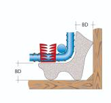
The Supo Duo is mounted on reinforcement cages in the stirrup corner area. It holds the concrete cover in two directions. Installation is possible on reinforcement  $\varnothing$  3-18 mm. The Supo Duo can also be supplied with 2 clamps as an option. Thanks to the specially designed clamp shape, the Supo clamps optimally to the reinforcing steel. Fast installation is guaranteed.
