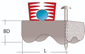
The mounting supo is used to fix the mounting reinforcement. The mounting supo is nailed to the formwork using the factory-fitted aluminum nail. The reinforcement bar ( $\varnothing$  3-18 mm) is simply inserted into the plastic clip. This enables the reinforcement to be set up quickly. Thanks to the specially designed shape of the clip, the Supo clamps optimally to the reinforcing steel.
