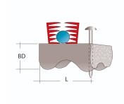
The mounting supo is used to fix the mounting reinforcement. The mounting supo is nailed to the formwork using the factory-fitted aluminum nail. The reinforcement bar (Ø 3-18 mm) is simply inserted into the plastic clip. This enables the reinforcement to be set up quickly. Thanks to the specially designed shape of the clip, the Supo clamps optimally to the reinforcing steel.
