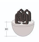
The poured concrete spacer has a round contact surface. The double clamp clamps well to the reinforcing steel. The spacer can be installed on both vertical and horizontal reinforcement. Installation is possible on reinforcement  $\varnothing$  6-16 mm.
