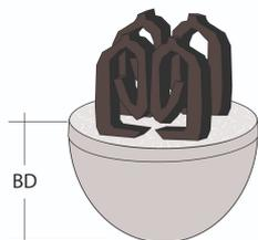
The poured concrete spacer has a round contact surface. The double clamp clamps well to the reinforcing steel. The spacer can be installed on both vertical and horizontal reinforcement. Installation is possible on reinforcement Ø 6-16 mm.
