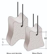
The Bipo with wire can be mounted on upright and horizontal reinforcement. The Bipo is manufactured with a flat contact surface as standard and can also be supplied with a trough on request. The Bipo is manufactured with an inserted black binding wire, which is also available in a galvanized version on request.
