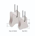
The Bipo with wire can be mounted on upright and horizontal reinforcement. The Bipo is manufactured with a flat contact surface as standard and can also be supplied with a trough on request. The Bipo is supplied with an inserted galvanized binding wire.
