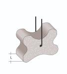
The Bipo bone with wire can be mounted on vertical and horizontal reinforcement. The bone shape allows three different concrete cover heights. The Bipo bones are supplied with an inserted galvanized binding wire.
