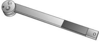
For inserting and removing tie rods.
