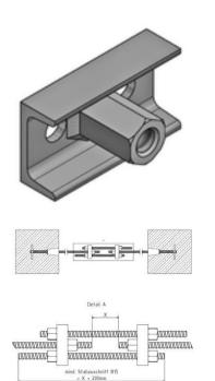
Turnbuckle B15 for connecting and pre-tensioning BETOMAX® tie rods.
