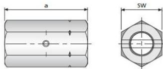
Made of machining steel, with stop pin, for extending tie rods. Compatible with Uni rods. Not usable for styrene!
