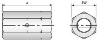
Made of machining steel, with stop pin, for extending tie rods. Comaptible with Uni rods. Not usable for styrene!
