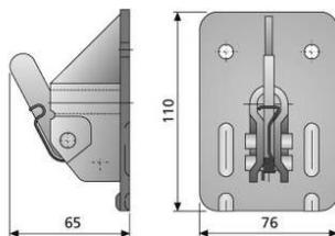
Reinforced, galvanized, with spring. For tension wire from 5 to 10 mm. Maximum load 10 kN for Ø 10 mm according to DIN 18216.
