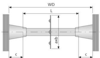
Water stop welded on Dist St-22 prevents the ingress of water. Use of FLUPP St plugs ensures that the steel tube is watertight. Conical holes can be filled with mortar or a concrete plug after removal of cones.
