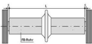
Swellable SD type water stop to prevent the ingress of water. Fitted using BETOMAX® SD installation pliers.
