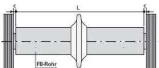
Swellable SD type water stop to prevent the ingress of water. Fitted using BETOMAX® SD installation pliers.
