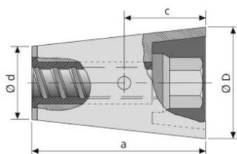
Metal-plastic cone for multiple use in concrete. Compatible with Uni-rods.
