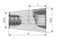
Metal-plastic cone for multiple use in concrete. Compatible with Uni-rods.
