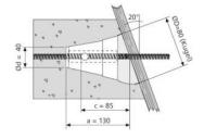
The MKK® Vario consists of a galvanized metal ring and a plastic spherical head. Due to its angle compensation of 20° the MKK® Vario can be used freely adjustable.
