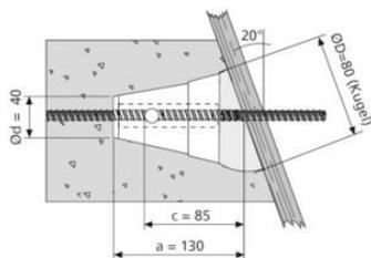
The MKK® Vario consists of a galvanized metal ring and a plastic spherical head. Due to its angle compensation of 20° the MKK® Vario can be used freely adjustable.
