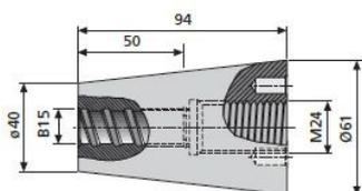
The SKK® BETOMAX 15 steel climbing cone is used in conjunction with the BETOMAX® 15 tie rod and a M 24 threaded bolt. It is used wherever the MKK® B 15 is selected as the positioning cone. The SKK® is tightened and released with the special SKK® spanner. Compatible with Uni15.
