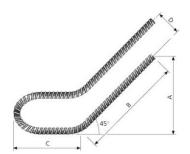
Made from weldable and bendable BETOMAX® tie rods 15, 20 and 26.5 For anchoring supports, for single-sided formwork Installed in first concreting section, in floor slab Can be extended with threaded connecting sleeve and MKK®
