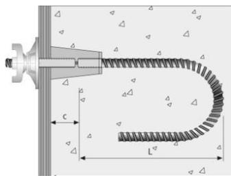
Made from weldable and bendable BETOMAX® tie rods 15, 20 and 26.5
