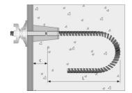
Made from weldable and bendable BETOMAX® tie rods 15, 20 and 26.5 Same applications as pigtail anchor, but also for smaller wall thicknesses
