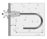
Made from weldable and bendable BETOMAX® tie rods 15, 20 and 26.5 Same applications as pigtail anchor, but also for smaller wall thicknesses
