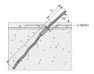
Made from weldable and bendable BETOMAX® tie rods 15, 20 and 26.5 For one-ended anchoring in concrete For use as lost (internal) tie rod Also for use in conjunction with cones, e.g. for climbing formwork
