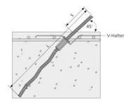
Made from weldable and bendable BETOMAX® tie rods 15, 20 and 26.5 For one-ended anchoring in concrete For use as lost (internal) tie rod Also for use in conjunction with cones, e.g. for climbing formwork
