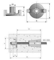
Casting, for one-sided anchoring. Max. load depends on the concrete quality and anchoring depth (Vt). Compatible with Uni 15.
