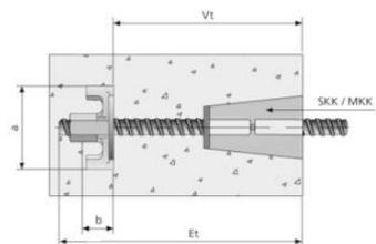
Casting, for one-sided anchoring. Max. load depends on the concrete quality and anchoring depth ( $Vt$ ). Compatible with Uni 15.
