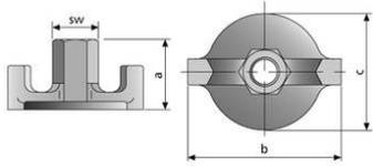
Casting, for one-sided anchoring. Max. load depends on the concrete quality and anchoring depth (Vt). Compatible with Uni 15.
