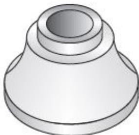
Casting for one-sided anchoring.
