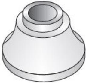
Casting for one-sided anchoring.
