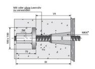
Made from an anchor plate with welded-on B 20 hexagon nut. For onesided anchoring. Compatible with Uni 20.
