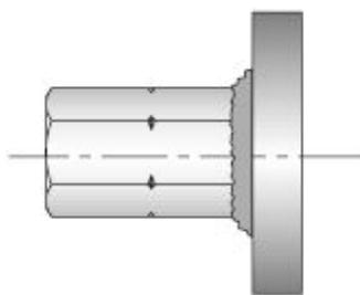
Made from an anchor plate with welded-on B 20 hexagon nut. For one-sided anchoring. Compatible with Uni 20.
