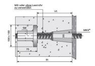
Made from an anchor plate with welded-on B 20 hexagon nut. For one-sided anchoring. Compatible with Uni 20.
