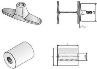
Forged weld-on part with fillet weld.
