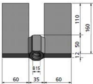
For welding at inclined areas, e.g. sheet pile walls.
