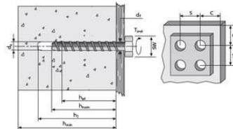
For securing push-pull props and BETOMAX® curb shuttering, galvanized.
