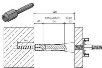
K-TEC-MS© from BETOMAX® systems is used for one-sided anchoring in existing concrete substrates.
