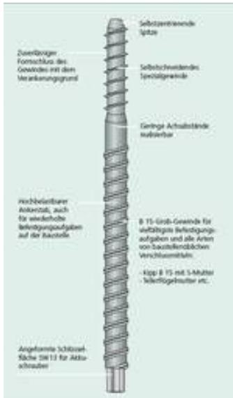
The BETOMAX® K-TEC-3s® can be reused several times and combines the benefits of a coarse thread for temporary machine fastening with those of a self-tapping concrete screw.
