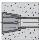
Extremely rugged cone for watertight resilient joints. The large contact surface area prevents pressure damage to the shuttering.
