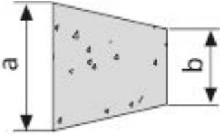
For closing tapered holes. Glued in with 2-component adhesive. 1 kg of adhesive is sufficient for approx. 60 concrete plugs.
