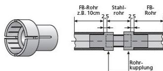
Plastic connecting piece for steel spacer tube 22 with fibrous concrete spacer tube (FB 22).
