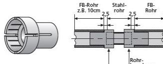
Plastic connecting piece for steel spacer tube 22 with fibrous concrete spacer tube (FB 22).
