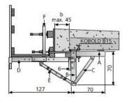
Standard application for regular ledges according to standard drawings issued by the German Federal Ministry of Transport, Construction and Housing.
