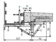
Standard application for regular ledges according to standard drawings issued by the German Federal Ministry of Transport, Construction and Housing.
