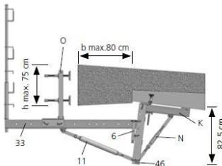
For wide cantilevered cap cornices in bridge construction.
