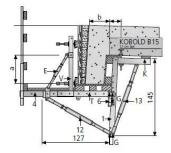
For overhanging, suspended decks with non-standard dimensions.
