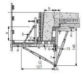
For overhanging, suspended decks with non-standard dimensions.
