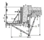
For overhanging, suspended decks with non-standard dimensions.
