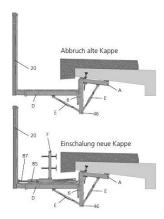
New renovation bracket with renovation ledger.
