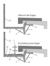
New renovation bracket with renovation ledger.
