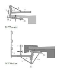
Console is folded onto the precast element during transport. After placing the precast element, just fold it over and it is immediately ready for use.
