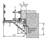
For narrow decks on ramps or wing walls and retaining walls.
