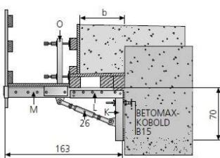
For large ledges on ramps or wing walls and retaining walls.
