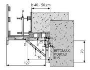
Can also be used for ramps or wing walls and retaining walls.
