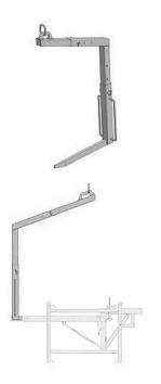
Crane mount to help assemble the pre-assembled cornice brackets.
