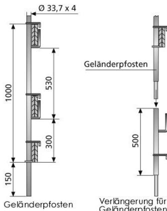
Complies with the safety rules for lateral protection and roof safety barriers as a means of safeguarding against falling (GB-I 807 of October 2002). According to DIN EN 12811.
